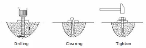
**Anchor Bolt:** 3/4" x 10" Long [Each bolt will provide 150 ft lbs of torque]
