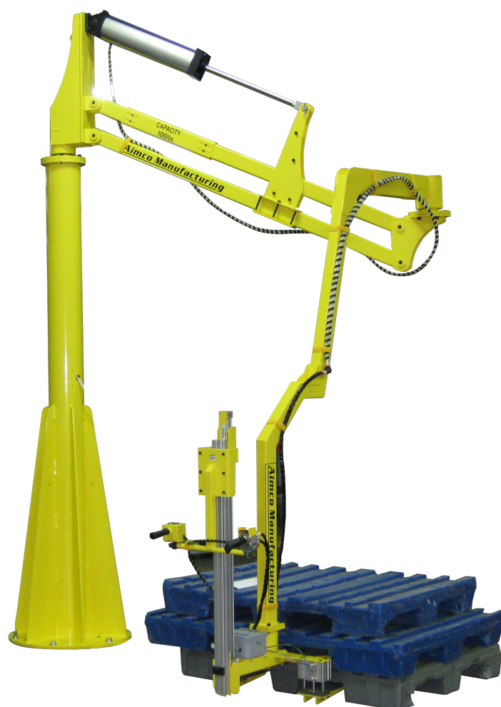
AIM5907 mounted to a pedestal + custom end effector with ergo handles
